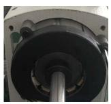
机定子 Install the Motor's Stator
