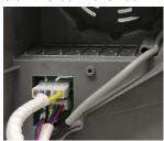
将电机上的电机动力线和电机霍尔线插到电控箱插头上,并将电控装到机器后端面上。 Put motor power cable and motor hall cable into controller'plug, then install the control box onto the back side of the machine.
