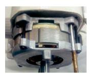
将电机定子的电线朝下装到机器后端面上,并用 3mm 内六角扳手拧紧 4 颗固定螺钉。 Put the power cable of motor stator down onto the back side of machine and tighten up 4 screws with 3mm hexagonal socket.
