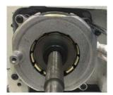
将电机定子的电线朝下装到机器后端面上,并用 4mm 内六角扳手拧紧 4 颗固定螺钉。 Put the power cable of motor stator down onto the back side of machine and tighten up 4 screws with 4mm hexagonal socket.
